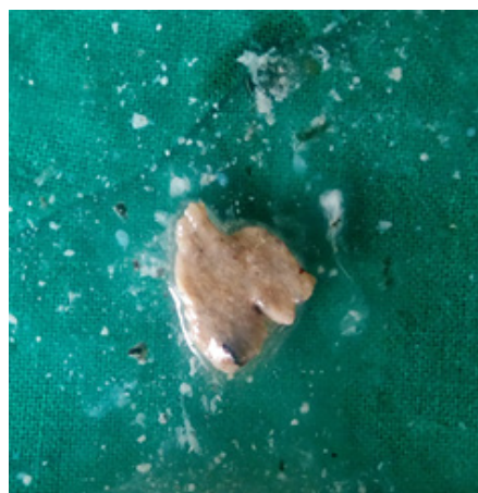
Figure. 6 White precipitation and Fragmentation of bone in H 2 SO 4 at 8 hours
